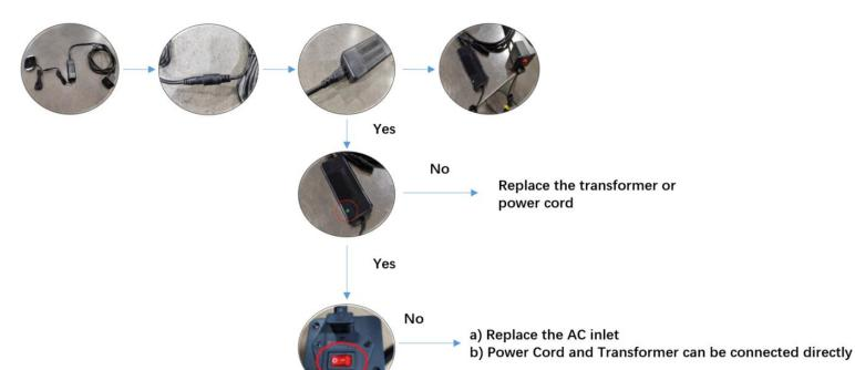
Step 2: Check whether the transformer light is on?
