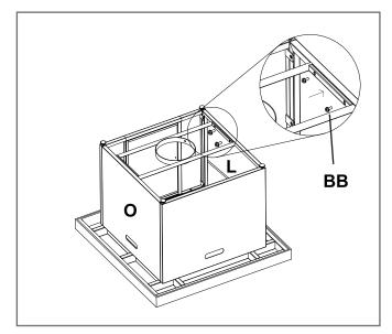
**5.** Using 1pc of M6\*35 bolt (CC), 1pc of ⊘6.5\*⊘16 Flat Washer (DD) and 1pc of M6 Nut (EE) to fix the control box by screwdriver (not included).
