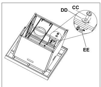
**6.** Place propane gas tank (not included) into the tank seat. Make sure the gas tank sits on the tank seat completely. Turn the preassembled wing screw on the outer part of tank seat clockwise to secure the propane gas tank tightly.
