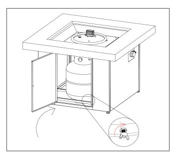
7. Turn the cylinder valve on the tank clockwise to close the propane tank. Attach the preassembled regulator from the table top to the cylinder valve by turning the regulator coupling nut clockwise. Make sure it is fastened securely and tighten connections by hand only.
