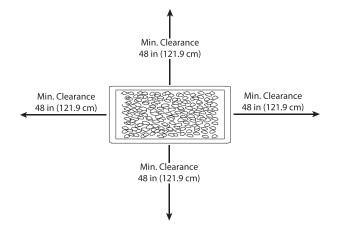
Combustible materials should not be within 72 inches of the top of the unit, or within 48 inches around the entire unit.
