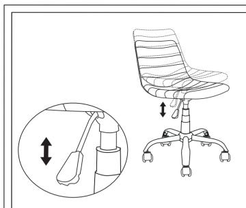
To adjust seat height — while seated, lean forward and reach under the right side of the seat to find the adjustment handle.
