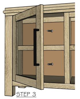
Reverse the position of the pull and tighten screws.
