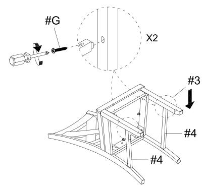
IMPORTANT: PRESS DOWN the Front legs (#3) when securing with side Stretchers (#4) using screws provided (#G) to avoid the gap between legs and stretchers.
